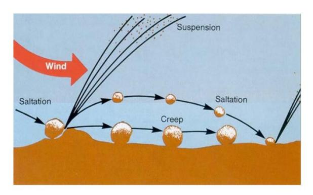
Saltating particles are primary disturbance leading to suspension
