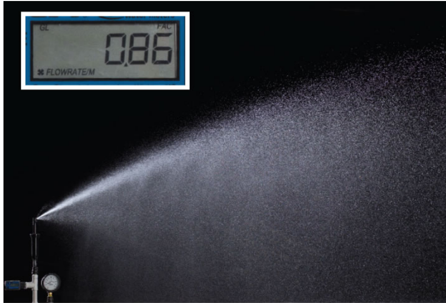
1800 Spray with PRS at 79 psi inlet pressure. PRS regulates flow to 0.86 gallons per minute.
