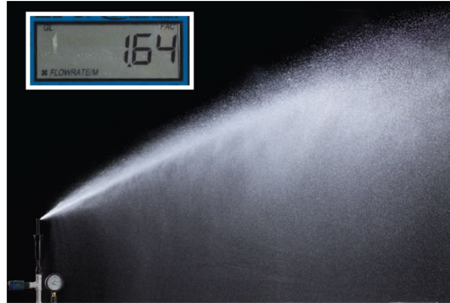
Non-PRS competitive spray at 79 psi inlet pressure. Without PRS, flow rises to 1.64 gallons per minute.
